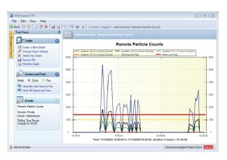
Graphs support control lines, linear/log axes and the right y-axis. Graphs can be zoomed and panned to better view their data. Graphs can be printed and exported to image files.
