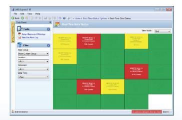
RT version, only - Real Time Data Status can display the alarm status of all recently collected data on one screen.
